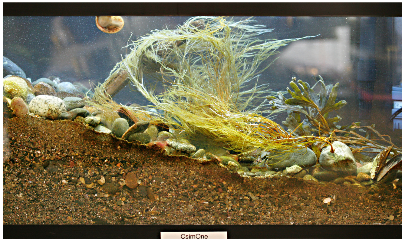
FIG 1 Bringing the environment into the laboratory. Image of a 76-l (20-gallon) aquarium for the incubation of marine sand biofilm bacteria in a simulated environment. The aquarium contains natural seawater, beach sand, flora, and invertebrate fauna from Canoe Beach, Nahant, MA. Operated in the laboratory of Kim Lewis at Northeastern University, the simulated environment is maintained with a filter system, a protein skimmer, a circulator, and regular exchanges of water freshly collected from the beach. This system can be used as an incubation environment, and the sand sediment can be used as a source of environmental bacteria.
