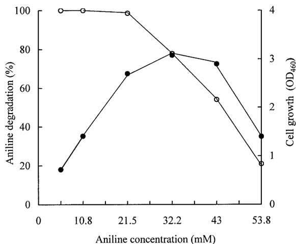
**Fig. 1** Effect of aniline concentration on its degradation and on the growth of *Delftia* sp. AN3. Experiments were conducted in 500-ml conical flasks containing 200 ml MMN media containing up to 53.8 mM aniline. Each flask was inoculated with 20  $\mu\text{l}$  of LB-cultured cells and incubated for 3 days at 30 °C with rotary shaking at 180 rpm. —○— Aniline degradation, —●— Cell growth
