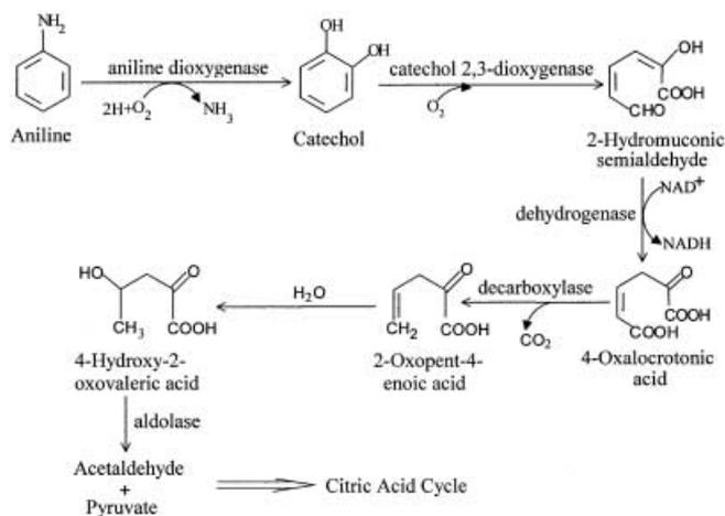
**Fig. 2** Proposed pathway of aniline degradation in *Delftia* sp. AN3
