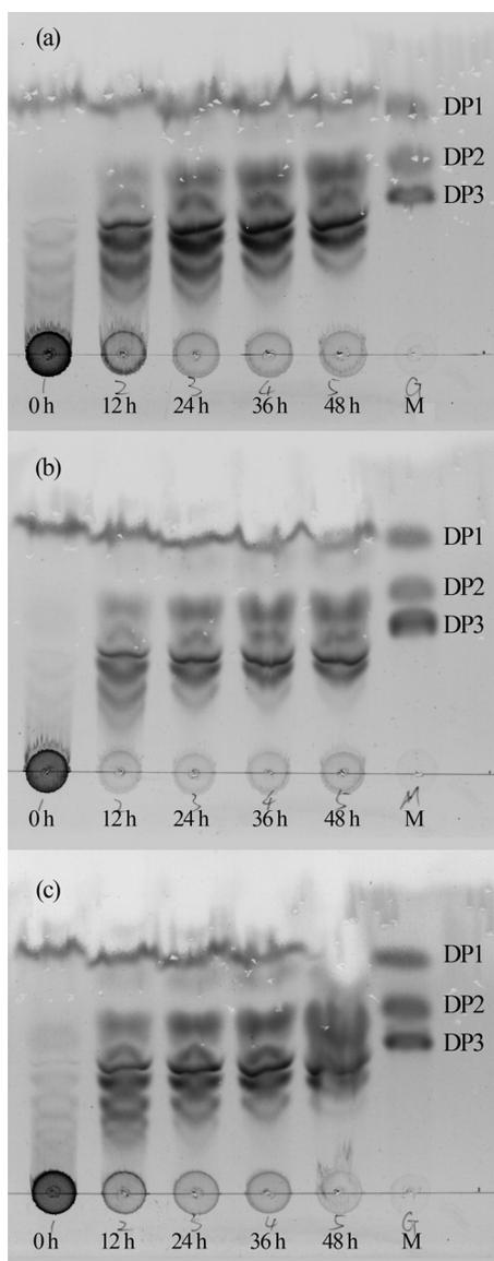
FIG 3 Thin-layer chromatograms of the products of sodium alginate, polymannuronic acid, and polyguluronic acid degradation by cALY, showing their substrate specificity. (a) Sodium alginate; (b) polymannuronic acid; (c) polyguluronic acid. DP, degree of polymerization.
